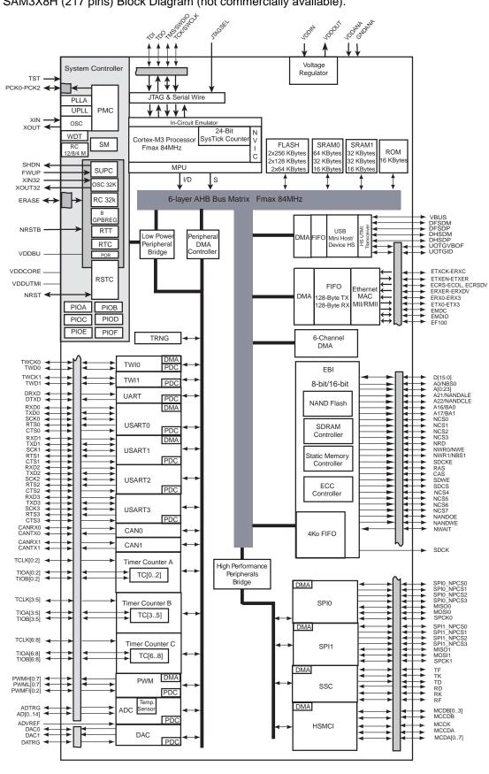
Figure 2-4. SAM3X8H (217 pins) Block Diagram (not commercially available).
