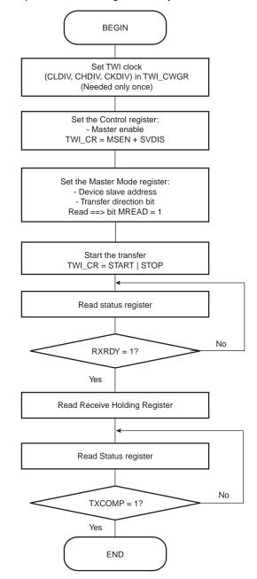
Figure 34-18. TWI Read Operation with Single Data Byte without Internal Address
