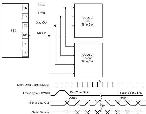
Figure 31-19. Time Slot Application Block Diagram
