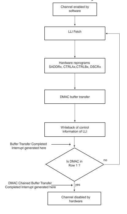
Figure 24-9. DMAC Transfer Flow for Linked List Source Address and Contiguous Destination Address
