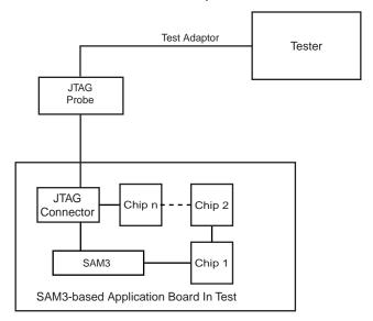
Figure 13-3. Application Test Environment Example
