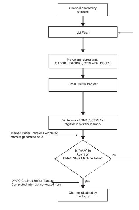
Figure 24-7. DMAC Transfer Flow for Source and Destination Linked List Address
