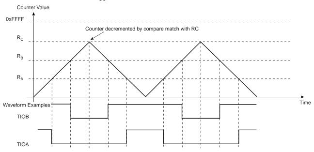
Figure 37-14. WAVSEL = 11 With Trigger
