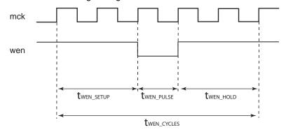
Figure 27-33. Write Enable Timing for NAND Flash Device Data Input Mode.
