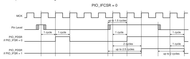
Figure 32-6. Input Debouncing Filter Timing
