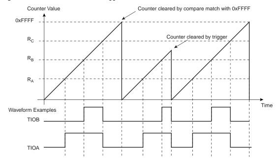
Figure 37-8. WAVSEL= 00 With Trigger
